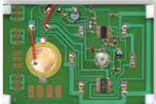
SM-200K PC board showing practice areas & mounted components
