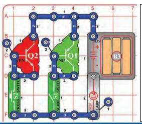
This circuit is similar to the preceding one except for the way the transistors are connected.
