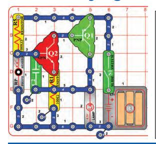
Turn on the slide switch (S1). If there is enough light on the photoresistor (RP), the lamp (L4) will not light. Place your finger over the photoresistor and now the lamp lights. The lamp will stay on until you turn off the slide switch. A simple mail notifying system can be made using this circuit.
