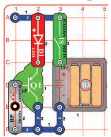
Turn on the slide switch (S1), the brightness of the LED (D1) depends on how much light shines on the photoresistor (RP).
