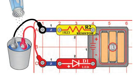
Place the jumpers in a cup of water as in the preceding project; the LED (D1) should be dimly lit. Slowly add salt to the water and see how the LED brightness changes, mix it a little so it dissolves. It will slowly become very bright as you add more salt. You can use this bright LED condition as a saltwater detector! You can then reduce the LED brightness by adding more water to dilute the salt.
