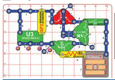
Set the adjustable resistor (RV) to the top position, turn the slide switch (S1) on and the speaker (SP2) sounds. Slowly adjust the adjustable resistor down; the loudness decreases and the time the sound is on is longer. Adjusting the lever down turns the NPN transistor (Q1) off, lowering the voltage on space war IC (U3).
