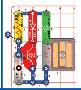
Turn on the slide switch (S1), the brightness of the LED (D1) depends on how LITTLE light shines on the photoresistor (RP). The resistance drops as more light shines, diverting current away from the NPN (Q2).
