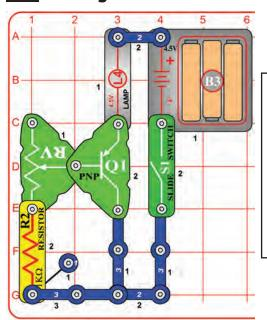
Compare this circuit to that in Project #60. The maximum lamp (L4) brightness is less here because the lamp resistance reduces the emitterbase current, which controls the emitter-collector current. The point on the PNP (Q1) that the lamp is now connected to (grid point C3) is called the emitter.
