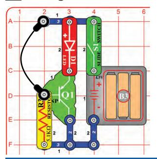
Build the circuit with the jumper connected as shown, and turn it on. Nothing happens. Break the jumper connection and the light turns on. You could replace the jumper with a longer wire and run it across a doorway to signal an alarm when someone enters.
