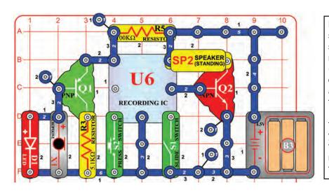
Build the circuit shown. Turn on the slide switch (S1), you hear a beep signaling that you may begin recording. Talk into the microphone (X1) up to 5 seconds, and then turn off the slide switch (it also beeps after the 5 seconds expires). Press the press switch (S2) for playback. It plays the recording you made followed by one of three songs. If you press the press switch before the song is over, music will stop. You may press the press switch several times to play all three songs.
