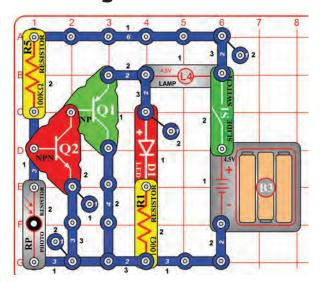
Turn the slide switch (S1) on. If there is light on the photoresistor (RP) then the LED (D1) turns on. Cover the photoresistor to switch off the LED and switch on the lamp (L4).
