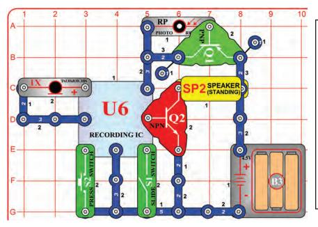
Build the circuit shown and press the press switch (S2). It plays a recording followed by one of three songs. Adjust the amount of light on the photoresistor (RP) to change the volume and alter the tone. Wave your fingers over the photoresistor for some cool sound effects.
