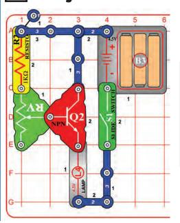
Compare this circuit to that in Project #61. It is the NPN transistor (Q2) version and works the same way. The same principles apply here as in Projects #60-#62, so you should expect it to be less bright than Project #62 but as bright as Project #61.
