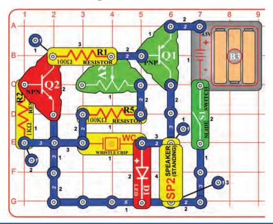
Build the circuit, turn it on, and move the setting on the adjustable resistor (RV). It makes a loud, annoying whine sound. The red LED (D1) appears to be on, but it is actually flashing at a very fast rate.
