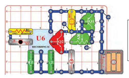
Build the circuit shown and press the press switch (S2). It plays a recording followed by one of three songs. Move the slider on the adjustable resistor (RV) around to change the volume and for some sound effects. You may press the press switch several times to play three songs. The lamp is used to limit the current and will not light.
