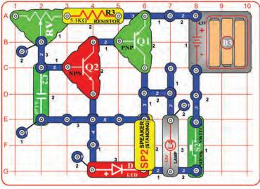
Build the circuit and set the adjustable resistor (RV) control lever to the left. When you press down on the press switch (S2) you will here a tone. By pressing and releasing the press switch you can generate long and short tones called Morse code. For International code, a short tone is represented by a "+", and a long tone by a "-". See the chart above for letter or number followed by code.
