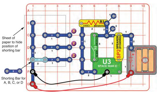
Build the circuit at left. It uses both jumper wires as permanent connections. It also uses two 2-snap wires as "shorting bars".
