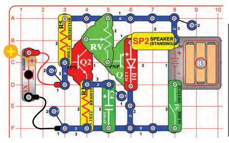
this Build audio amplifier circuit shown. Set the adjustable resistor (RV) control lever to the bottom position. Set the slide switch (S1) on and blow into the microphone (X1). You should hear static on the speaker (SP2) and the LED (D1) may flicker.
