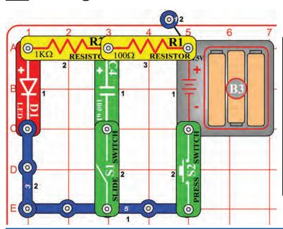
Build the circuit, turn on the slide switch (S1), and press the press switch (S2). You see that the LED (D1) doesn't turn off immediately after you release the switch. If you remove the capacitor from the circuit by turning off the slide switch, then the LED goes off immediately.
