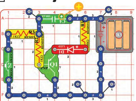
LED gradually brightens. Now release the press switch. The capacitor begins to discharge, sending input current to the transistor. As the capacitor discharges, the input current reduces to zero and gradually turns off the LED and the transistor.
