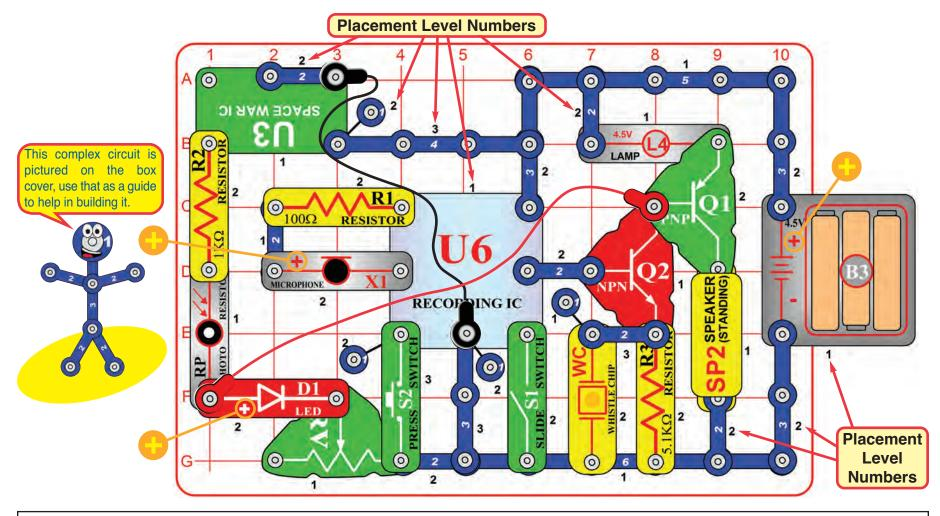
Circuit Maker Sound Plus 200 uses electronic blocks that snap onto a clear plastic grid to build different circuits. These blocks have different colors and numbers on them so that you can easily identify them.
