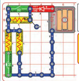
Build the circuit and turn on the slide switch (S1), the LED (D1) will be lit. To increase the LED brightness, turn on the press switch (S2). To decrease the LED brightness, turn off the slide switch.
