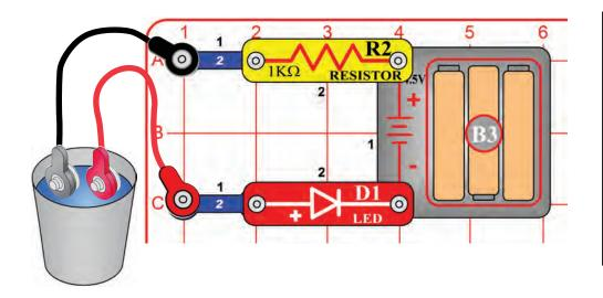
Build the circuit at left and connect the two jumpers to it, but leave the loose ends of the jumpers lying on the table initially. The LED (D1) will be dark because the air separating the jumpers has very high resistance. Touch the loose jumper ends to each other and the LED will be bright, because with a direct connection there is no resistance separating the jumpers.
