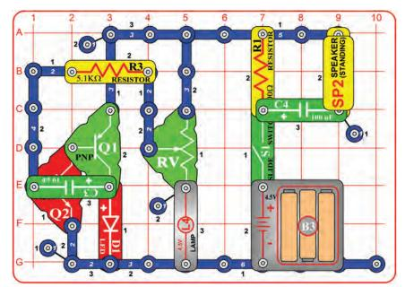
Turn on the slide switch (S1) and slowly move the adjustable resistor (RV) control lever until the red LED (D1) is flashing. The speaker (SP2) will also make a clicking sound. The lamp (L4) will not light.
