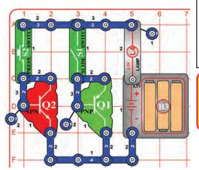
The press switch (S2) controls the NPN transistor (Q2) and can turn on the lamp. The slide switch (S1), however, cannot control the PNP transistor (Q1) and so cannot turn on the lamp.
