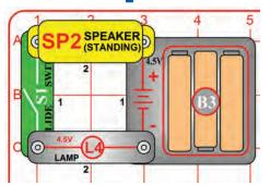
Turn the slide switch (S1) on and off several times. You hear static from the speaker (SP2) when you first turn on the switch, but hear nothing after it is left on.
