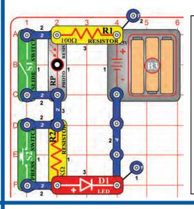
Turn on either or both switches (S1 & S2) and compare the LED (D1) brightness.
