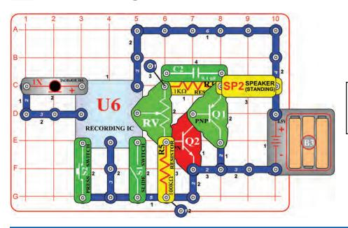
This circuit uses the variable resistor (RV) as a volume control. Build the circuit and set RV to the middle position. As the music plays, you can adjust the volume by moving RV control up or down from the center position.
