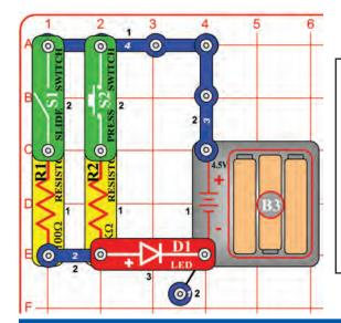
Turn on either or both switches (S1 & S2) and compare the LED (D1) brightness.
