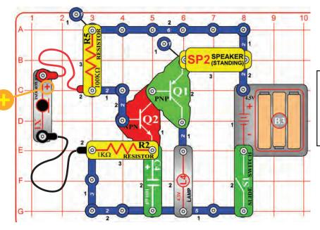
Build this audio amplifier circuit shown. Set the slide switch (S1) on and blow into the microphone (X1). You should hear static on the speaker (SP2).
