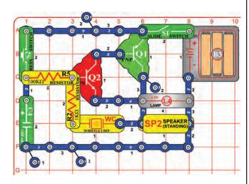
Build the circuit on the left; note that there is a 4-snap wire on layer 1 that is not connected to a 3-snap wire that runs over it on layer 3. Turn on the slide switch (S1), then press and release the press switch (S2). There is a doorbell sound that slowly fades away.
