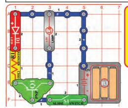
Transistors use a small current to control a large current, and have three connection points (the small current, the larger current, and the combined current). But they are actually constructed using two diodes that are connected together. These diodes are similar to your LED (light emitting diode) except that they don't emit light.
