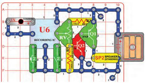
This circuit uses the variable resistor (RV) as a volume control. Build the circuit and set RV to the middle position. As the music plays, you can adjust the volume by moving RV control up or down from the center position.
