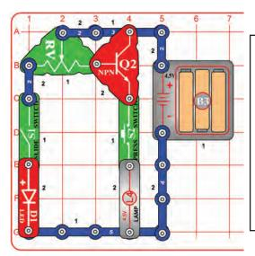
Turn on the circuit using the slide switch (S1) and/or the press switch (S2) and move the adjustable resistor's (RV) control lever around to adjust the brightness of the D1 and L4. When the adjustable resistor is set to one side, that side will have low resistance and its light turns (assuming the switch on that side is ON) on while the other is OFF.
