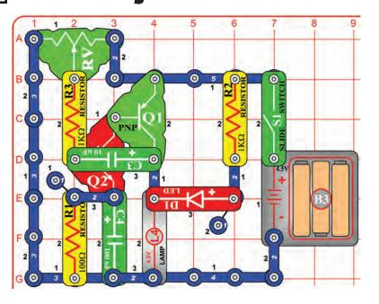
Turn on the slide switch (S1) and slowly move the lever on the adjustable resistor (RV) until both the lamp (L4) and LED (D1) are flashing. They will only flash together over a narrow range of the lever setting.
