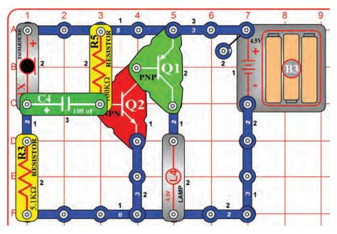
Install the parts. The lamp (L4) will be on. It will be off as long as you blow on the microphone (X1).
