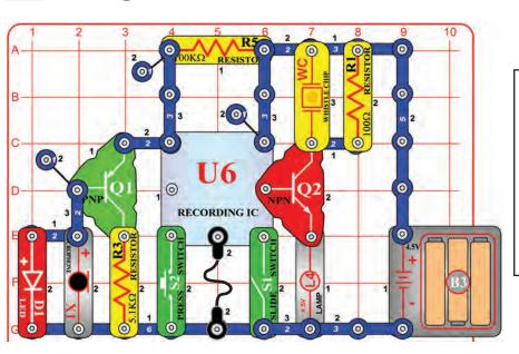
Build the circuit shown. Turn on the slide switch (S1), you hear a beep signaling that you may begin recording. Talk into the microphone (X1) up to 5 seconds, and then turn off the slide switch (it also beeps after the 5 seconds expires). Press the press switch (S2) for playback. It plays the recording you made followed by one of three songs. The lamp (L4) will not light.
