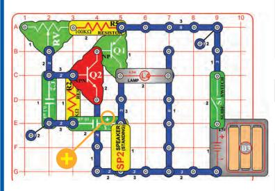
Set the adjustable resistor (RV) to the far left and turn on the slide switch (S1). The LED (D1) lights and the speaker (SP2) sounds once per second. Adjusting the adjustable resistor to the right increases the rate.
