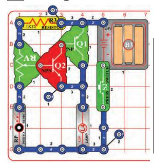
Press the press switch (S2) on and set the adjustable resistor (RV) so the lamp (L4) just lights. Slowly cover the photoresistor (RP) and the lamp brightens. If you place more light at the photoresistor the light dims.
