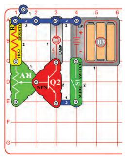
Compare this circuit to that in Project #60, it is the NPN transistor (Q2) version and works the same way. Which circuit makes the lamp (L4) brighter? (They are about the same because both transistors are made from the same materials).
