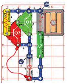
Build the circuit with the jumper connected as shown, and turn it on. Nothing happens. Break the jumper connection and the lamp (L4) turns on. You could replace the jumper with a longer wire and run it across a doorway to signal an alarm when someone enters.
