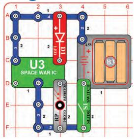
When there is light on the photoresistor (RP), its resistance is low and the LED (D1) will flicker. Shield the photoresistor from the light; the LED should turn off.
