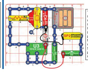
Turn on the slide switch (S1), the whistle chip (WC) sounds and D1 and L4 light. The whistle chip (WC) and LED are in parallel. To connect the speaker in parallel with the lamp press S2. Now you have two parallel circuits connected in series.
