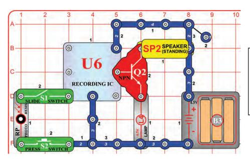
You will only hear music if you turn on the slide switch (S1) <u>AND</u> press the press switch (S2) <u>AND</u> there is light shining on the photoresistor (RP). This is referred to as an AND gate in electronics. The lamp (L4) is only used to limit current and will not light.
