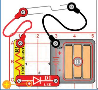
Build the circuit, but leave the ends of the red and black jumper wires unconnected at first.
