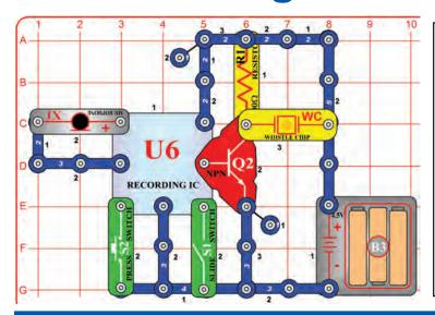
Build the circuit shown. Turn on the slide switch (S1), you hear a beep signaling that you may begin recording. Talk into the microphone (X1) up to 5 seconds, and then turn off the slide switch (it also beeps after the 5 seconds expires). Press the press switch (S2) for playback. It plays the recording you made followed by one of three songs. If you press the press switch before the song is over, music will stop. You may press the press switch several times to play all three songs.
