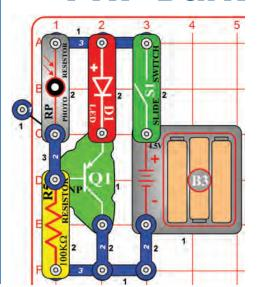
Turn on the slide switch (S1), the brightness of the LED (D1) depends on how LITTLE light shines on the photoresistor (RP). The resistance drops as more light shines, so more current gets to the  $100 \mathrm{k}\Omega$  resistor (R5) from the photoresistor path and less from the PNP-diode path. This is similar to the NPN circuit above.
