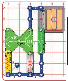
Build the circuit and vary the lamp (L4) brightness with the adjustable resistor (RV), it will be off for most of the resistor's range. The point on the PNP (Q1) that the lamp is connected to (point E3 on the base grid) is called the collector, hence the name for this project.
