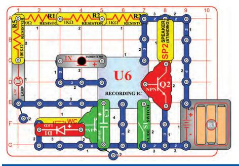
Build the circuit shown. Tap the case of the red LED (D1) for playback. It plays the recording you made followed by one of three songs. If you tap the case during playback, the music stops. The lamp (L4) and red LED do not light in this project. The lamp function as a jumper and the red LED as a diode.
