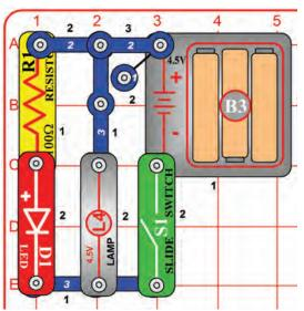
Turn on the slide switch (S1) and the LED (D1) and lamp (L4) light. If one of the them is broken then the other will still be on, because they are in parallel. An example of this is most of the lights in your house; if a bulb is broken on one lamp then the other lamps are not affected.
