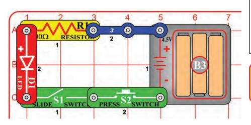
Build the circuit shown. Notice that if you turn on the slide switch (S1) AND press the press switch (S2) the LED (D1) lights up. Once again, there is no partially lit state here, the LED is either totally on or totally off. Two switches like this may be used to turn on the same light in your house, the room switch and the master switch in the electrical box. You could also have more than two switches and the circuit would function the same way.
