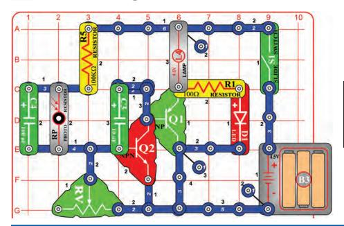
Turn the slide switch (S1) on. Set the adjustable resistor (RV) so that the lamp (L4) is on when there is light on the photoresistor (RP), and the LED (D1) is on when you cover the photoresistor.
