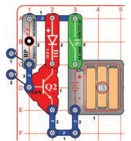
Turn on the slide switch (S1), the brightness of the LED (D1) depends on how much light shines on the photoresistor (RP). The resistance drops as more light shines, allowing more current to the NPN (Q2).
