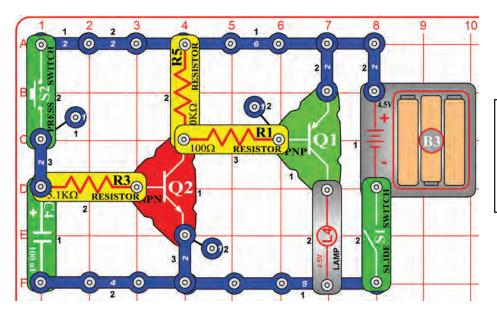
Turn on the switch and press the press switch (S2). The lamp (L4) stays on for a few seconds after you release the press switch.
