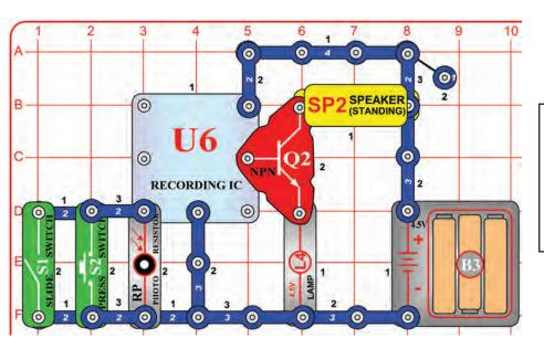
You will hear music if you turn on the slide switch (S1)  $\underline{OR}$  press the press switch (S2)  $\underline{OR}$  there is light shining on the photoresistor (RP). This is referred to as an OR gate in electronics. The lamp (L4) is only used to limit current and will not light.
