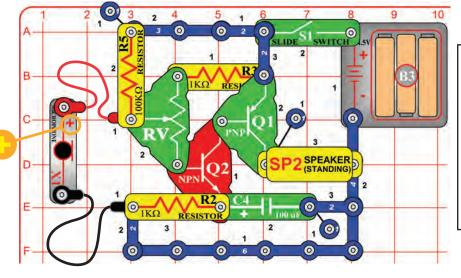
Build this audio amplifier circuit shown. Set the slide switch (S1) on and talk or blow into the microphone (X1). You should hear your voice on the speaker (SP2). Your voice will not be very loud. Control the volume by adjusting the RV control.
