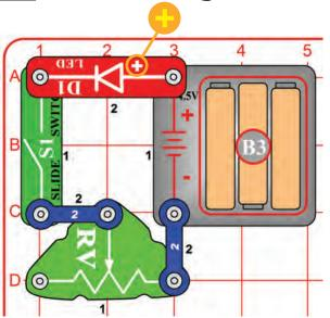
In this circuit, changing the adjustable resistor (RV) setting changes the brightness of the LED (D1).
