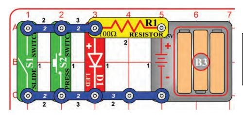
Build the circuit at left and test the combinations of the slide switch (S1) and press switch (S2). If you compare it to the OR circuit in Project #32, you can see the LED (D1) lights in the opposite combinations of that circuit. Hence, we refer to it as a <u>NOR</u> circuit (short for "NOT this OR that"). Like the OR and AND, it is an important building block in computers.
