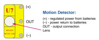
All objects (including people and animals) produce infrared radiation due to the heat in them. Infrared radiation is similar to visible light but has a longer wavelength that our eyes cannot detect. The lens on top of the motion detector module filters and focuses the radiation, it is most sensitive to the radiation produced by our bodies.
