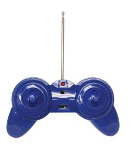
The Remote Control Unit (in all Snap Rover models) contains a radio transmitter circuit, a specialized radio encoder integrated circuit (W55RFS27T3B or equivalent), and other supporting components. Its actual schematic is complex and looks like this:
