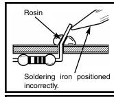
2. Insufficient solder - let the solder flow over the connection until it is covered.
