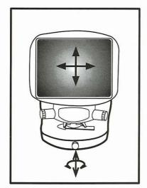
Rotate the bulb-positioning knob to adjust the illuminating area on the screen.
