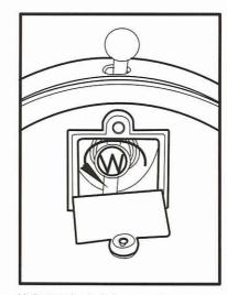
Unfasten the bulb in a counterclockwise direction.
