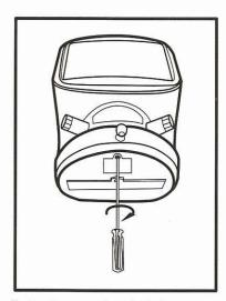
Fasten the screw in a clockwise direction.
