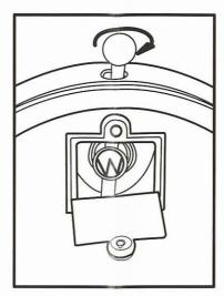
Rotate the bulb-positioning knob so that the bulb can be accessed.
