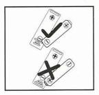
Make sure battey is inserted with the correct polarity.
