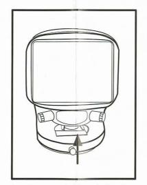
Insert a prepared slide under the stage clip.
