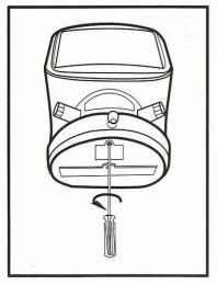
Unfasten the screw at the bulb compartment in a counter-clockwise direction.
