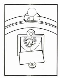
Turn the bulb upwards by rotating the bulb-positioning knob.
