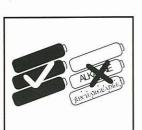
Only batteries of the same or equivalent type are to be used. Do not mix alkaline, standard (zinc carbon), or rechargeable (nickel cadmium) batteries.
