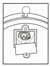
Fasten the bulb in a clockwise direction.
