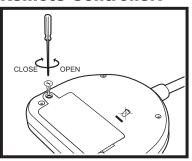
1) Open or close the cover with a philips screwdriver.
