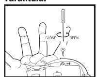
1) Open or close the cover with a philips screwdriver.
