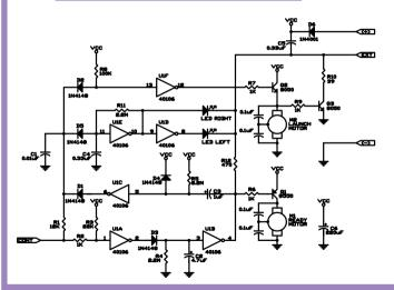
The **Disc Launcher unit** (only in SCROV-50 Deluxe Snap Snap Rover) contains a complex electronic circuit to control when the loading and launching motors start up and shut down, and to flash the lights in the "eyes". Its schematic is shown at left.
