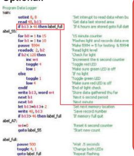
The data is stored in the same memory area as the main program with the write command, and retrieved by using a subroutine and the read command. When the press switch is pressed an interrupt stops the main program to execute the subroutine to retrieve the data stored thus far and send it to the terminal window. More details on how these commands work can be found under the Help menu at Snap Circuits® XP™.
