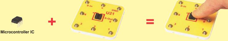
8-pin socket on Snap Circuits® platform
