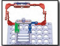
Place the parts on the base grid, then assemble the parts on the vertical snap wires (V1).
