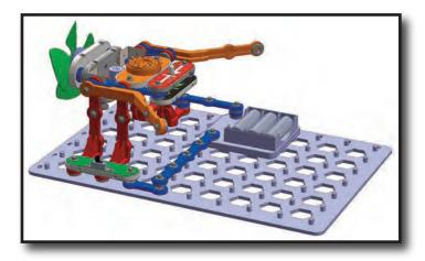
Place the parts on the base grid, then assemble the parts on the four 90 degree vertical snap wires (V1).
