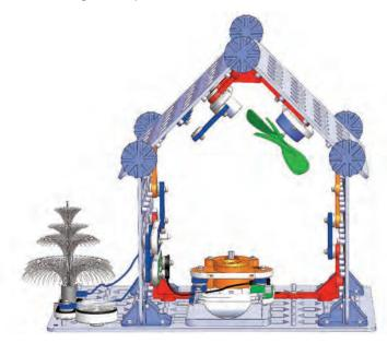
Turn on the slide switch (S1). The clear motor (M4) spins a ceiling fan, the lamp (L4) lights, the blink red LED (D11) lights, the color LED (D12) lights up the fiber optic festive tree, the orange motor (M9) spins the mirror ball, and the melody IC (U32) makes sound. Gently spin the magnet with your finger; the compass needle should follow it. Push the magnet near the reed switch (S9) and the blue LED (D9) lights.
