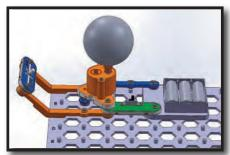
Build the circuit as shown; it has the blue LED (D9) mounted on two 45 degree vertical snap wires (V2). Place the mirror ball on the orange motor (M9).
